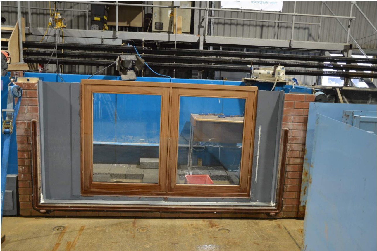
Figure 1.1: The Flood Company flood windows in the HR Wallingford test rig
