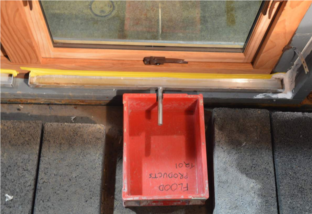
Figure 1.2: View from inside test rig showing drip tray and collection tank under the opening window.
