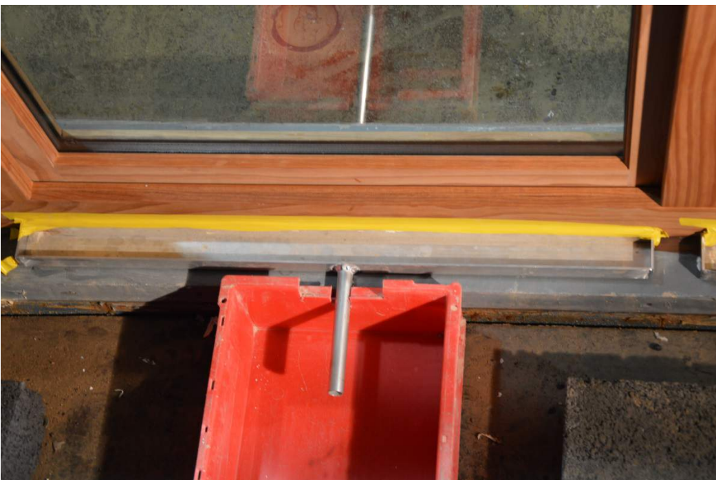
Figure 1.3: View from inside test rig showing drip tray and collection tank under the non-opening window
